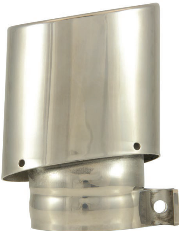
Figure 2 Re-designed, printed and post-processed tail pipe blend of sports car Porsche GT2 RS
