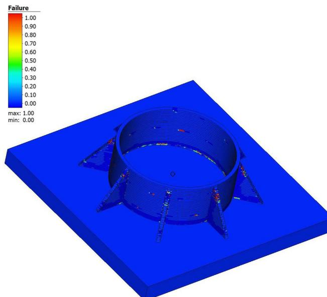
Figure 4: User-defined field of failure probability criterion, showing the vulnerable areas.
