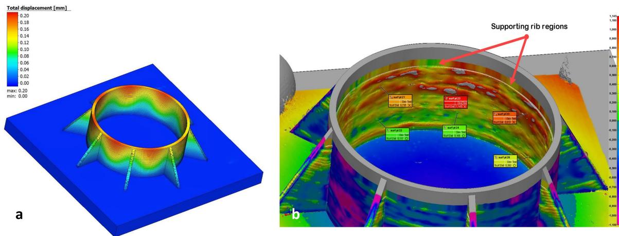
Figure 2: (a) Calculated displacement field, showing how the material is deformed under the given tool path and (b) comparison between the nominal CAD dimensions and the 3D-scanned geometry after deposition.
