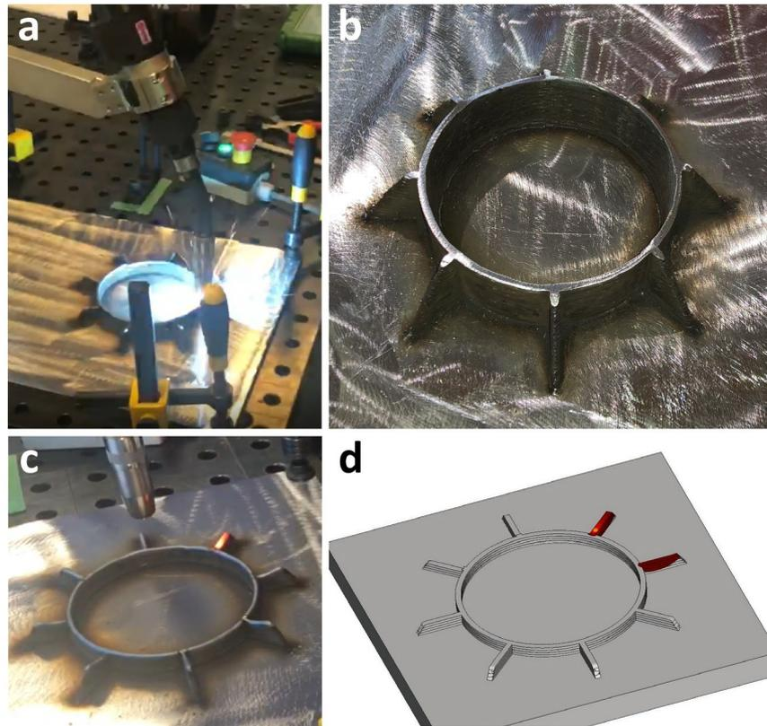
Figure 5: (a) WAAM deposition of the geometry, (b) the geometry after deposition, (c, d) a comparative image from the actual deposition and the numerical simulation results, showing the temperature field distribution.
