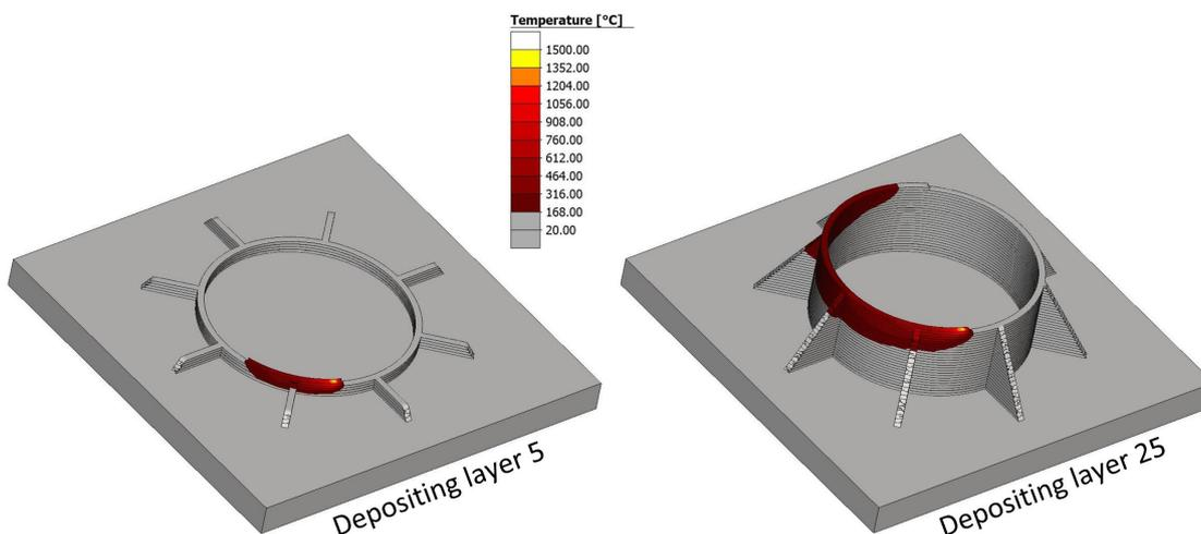
Figure 1: Temperature field comparison when the 5<sup>th</sup> layer and the 25<sup>th</sup> layer are being deposited.
