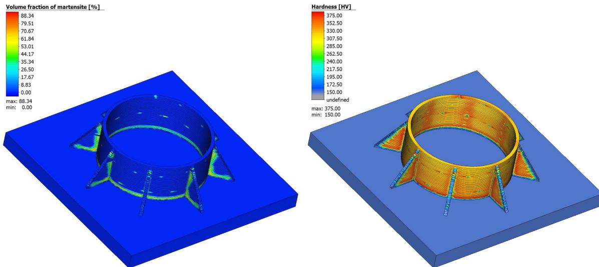
Figure 3: Martensite volume fraction and the estimated hardness profile, calculated based on the CCT data of the material.
